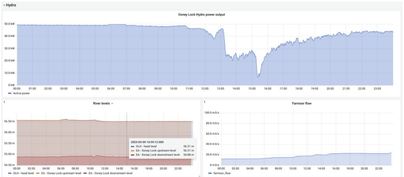
Figure [16]: PPS 2.0 dashboard showing historical generation data for the hydro and river conditions (Osney Lock Hydro)
