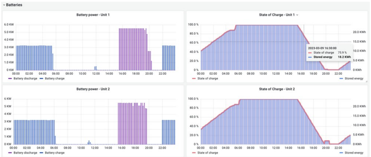
Figure [18]: PPS 2.0 dashboard showing the cycles of charge and discharge for each of the two batteries, as well as state of charge (%) and amount of energy stored (Osney Lock Hydro)
