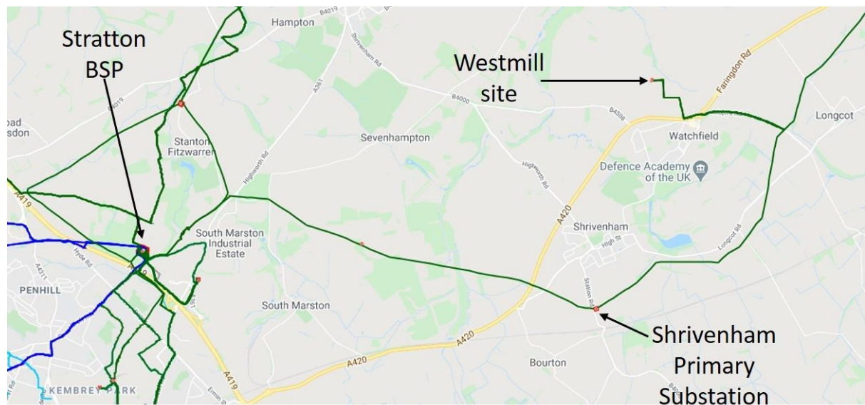
Figure 15: Relationship between the Westmill site, the primary substation, and the Bulk Supply Point
