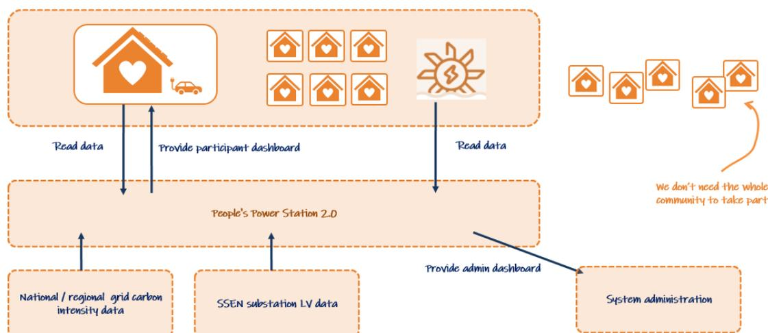
Figure 3: Data feeding into the Smart Community Energy System dashboard in Osney Supercharge
