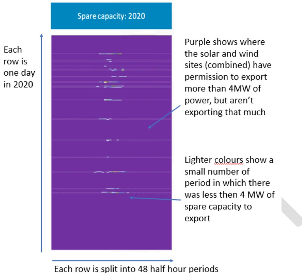
Figure 9: Capacity profile diagram for the solar and wind farms at Westmills
