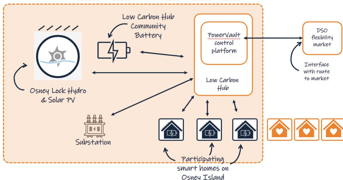
Figure 2: Osney Supercharge – overview of energy system behind a single secondary substation, linking into flexibility markets
