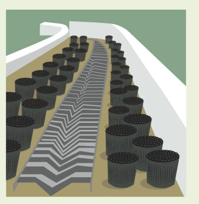
The fish pass is an innovative design by Dr Reinhard Hassinger from the University of Kassel, Germany. It's the first of its kind in the UK with the novel design combining concrete and naturalised sections, a resting pool and spawning grounds.
